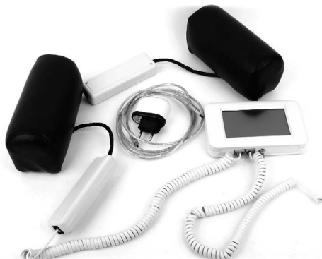
Figure 14 Final look of the set for acquisition, processing, numerical and graphical display of measurement values
