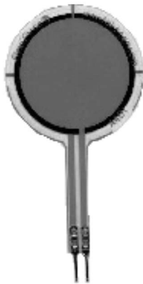
Figure 5 FlexiForce resistive force sensor, model A401 (manufacturer Tekscan, USA)
